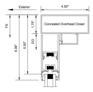
Series 900 Hinged Door - Swing Out - Medium Stile - Thermally Broken - Conceled Overhead Closer - Equal Leg Block Frame
