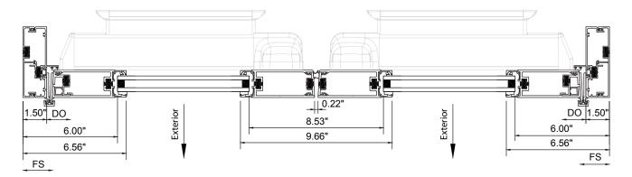
Series 900 Hinged Pair Door - Swing Out - Medium Stile - Thermally Broken - Equal Leg Block Frame
