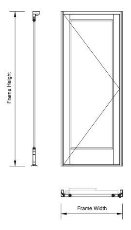
Series 900 Hinged Door - Swing Out - Medium Stile - Thermally Broken - Conceled Overhead Closer - Equal Leg Block Frame
