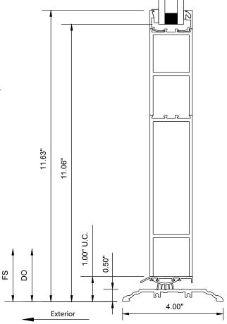
Series 900 Hinged Door - Swing Out - 10" Bottom Rail - Commercial Threshold
