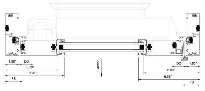
Series 900 Hinged Door - Swing Out - Medium Stile - Thermally Broken - Equal Leg Block Frame
