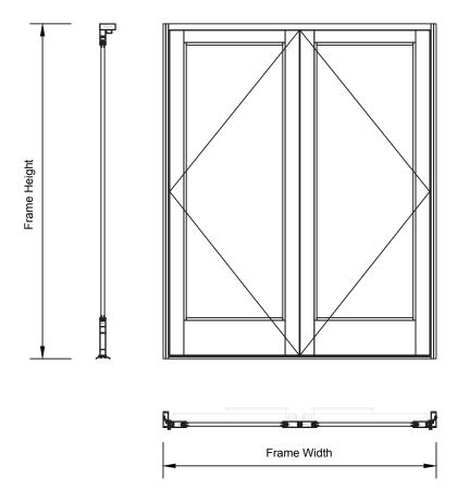
Series 900 Hinged Pair Door - Swing Out - Medium Stile - Thermally Broken - Conceled Overhead Closer - Equal Leg Block Frame
